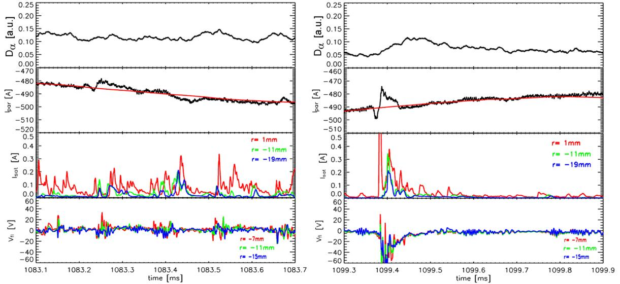
**Figure 3.** Temporal evolution of (from top to bottom)  $D_\alpha$  radiation, parallel electric current  $I_{par}$ , Ion saturation current  $I_{sat}$  at different radii, and Floating potential  $V_{fl}$  at different radii during the L-mode (left) and ELM (right).
