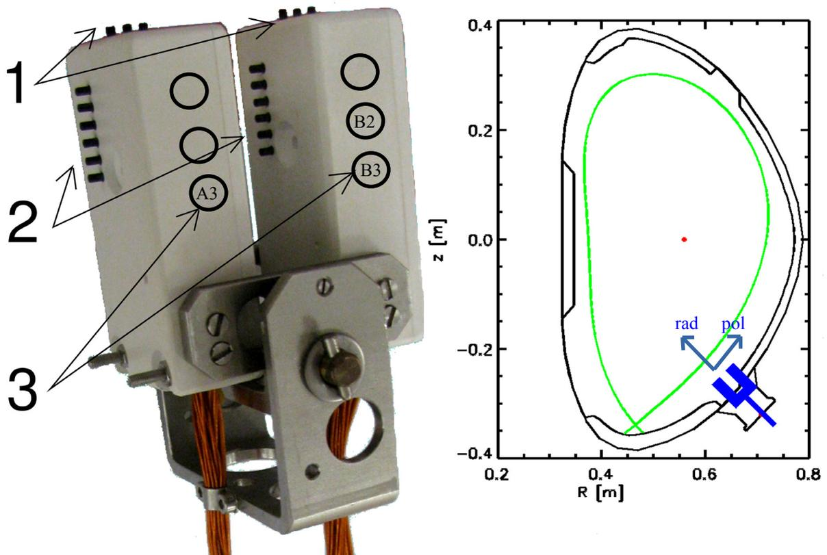
**Figure 1.** Left — Photographs of the U-probe (1—Triple probes, 2—rake probes, 3—coil sets hidden inside the probe head), right — schematic drawing of U-probe (blue) position inside the COMPASS tokamak with signed poloidal and radial direction (green line represents separatrix during the flat-top phase).
