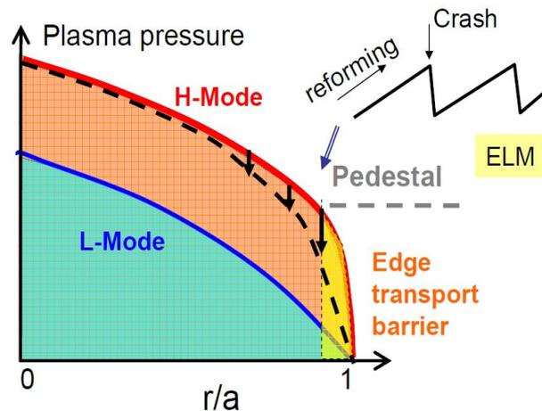
**Figure 2.** Schematic drawing of the H-mode regime and ELM creation.
