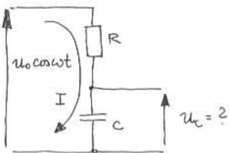
$$\bar{I} = \frac{\bar{u}}{\bar{Z}} \quad ; \quad \bar{Z} = \bar{Z}_R + \bar{Z}_C \quad ; \quad \bar{u} = u_0$$
