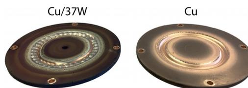
FIG. 2. Photograph of the utilized Cu/37W (left) and pure Cu (right) 3 in. targets used in the gas aggregation source. The pure W target is not shown.
