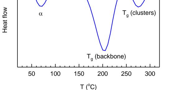
DSC curve for dried Nafion. The endothermic peak with maximum at 68°C which agrees well with the  $\alpha$ transition temperature determined by LT spectroscopy. The two endothermic processes occurring in the temperature range 150-235°C and 250-300°C can be attributed to glass transitions occurring in the polymeric PTFE backbone and inside the ionic clusters, respectively.
