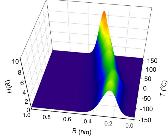
Thermal development of the free volume size distribution H(R) in Nation, where R is the free volume hole radius, calculated from LT results using the Tao-Eldrup model [6,7].
