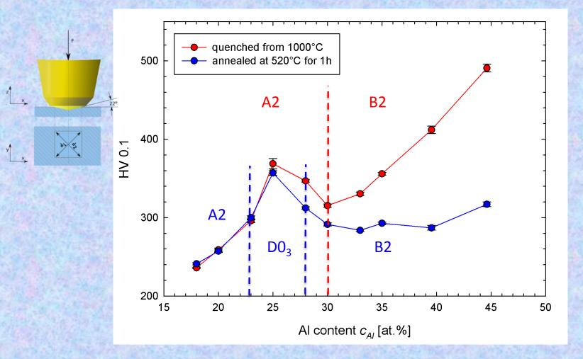
Measurable effect of vacancy hardening starts from  $c_{AI} > 25 \%$
