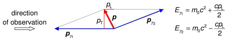
**Fig. 1.** Kinematical diagram of two-photon annihilation process (1) in a laboratory frame. The  $e^+ - e^-$ -pair brings total momentum vector  $\mathbf{p}$  with longitudinal and transversal components  $p_L$  and  $p_T$ , respectively. This causes a Doppler shift in energy of annihilation photons,  $E_{\gamma_1}$  and  $E_{\gamma_2}$ , with respect to electron/positron rest-mass energy  $m_0 c^2$ .
