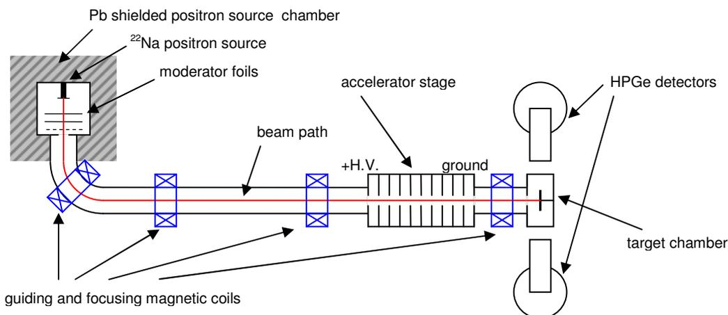
**Fig. 5.** Principal scheme of a magnetically guided slow-positron beam with variable energy.
