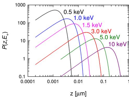
**Fig. 4.** Implantation profiles of monoenergetic positrons in Cu. Energies are inserted in the figure.
