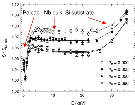
**Fig. 6.** Selected  $S(E)$  curves for the virgin Nb film and the Nb film loaded to various concentrations of hydrogen,  $x_H$  [at.<sup>-1</sup>].
