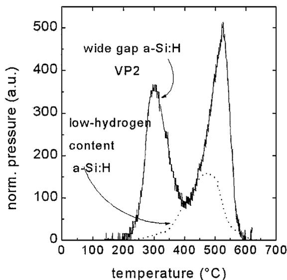
Figure 4. Comparison of a typical thermal desorption curve (normalized hydrogen pressure) of wide gap a-Si:H (solid line) with that of a-Si:H with low hydrogen content (dotted line).
