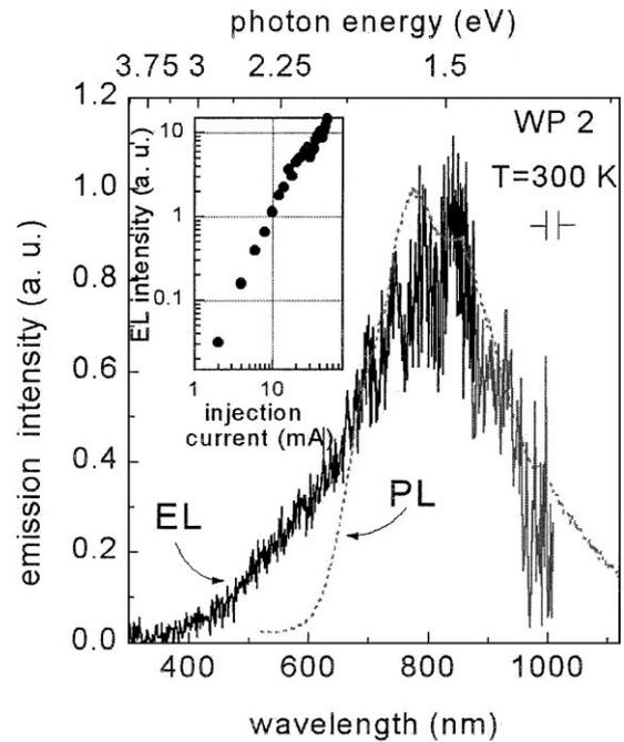
Figure 3. Comparison of the p-i-n EL emission spectrum (reverse bias 11 V, 40 mA—solid curve) with the PL emission spectrum of a relevant i-layer (dotted curve). Inset shows integral EL intensity as a function of the injection current.
