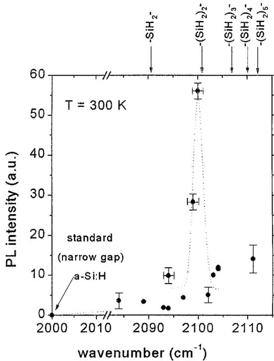
Figure 2. Integral PL intensity as a function of the frequency of the IR vibration mode in the vicinity of  $2100\text{ cm}^{-1}$  for the set of investigated samples. The dotted line is a guide for the eye.
