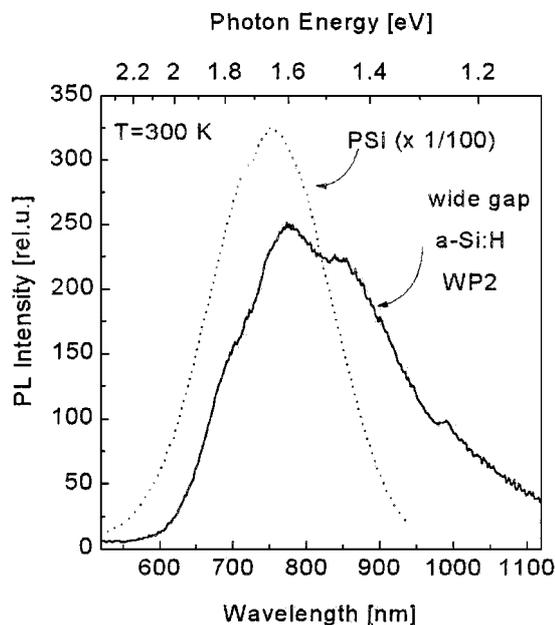
Figure 1. Comparison between PL spectra of wide gap a-Si:H (solid line) and a typical porous Si sample (dotted line).
