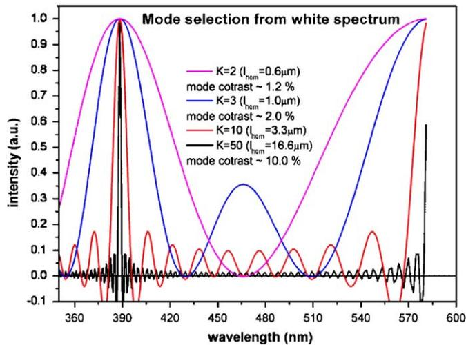
Fig. 3. Mode selection simulation for an ideally white spectrum, calculated for several values of  $l_{\text{hom}}$ . Spectra are normalized.
