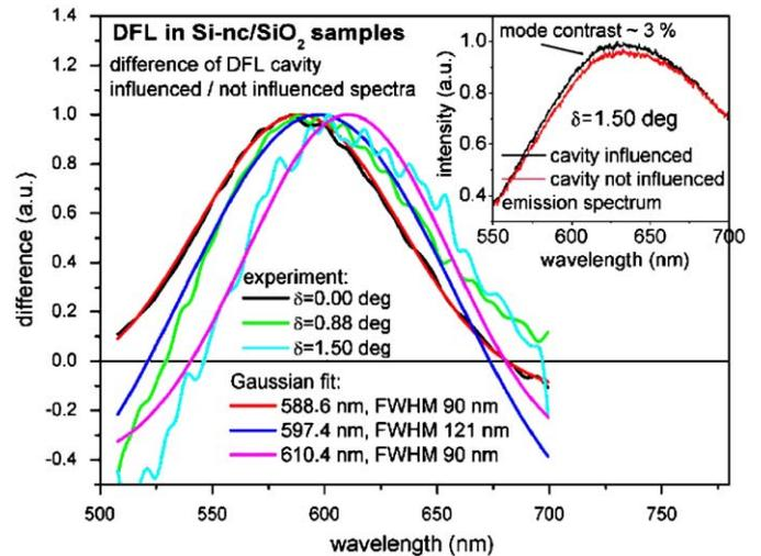
Fig. 4. Experimentally observed DFL modes excited in Si-nc/SiO<sub>2</sub>-based material. Curves are fitted by Gaussian shapes.
