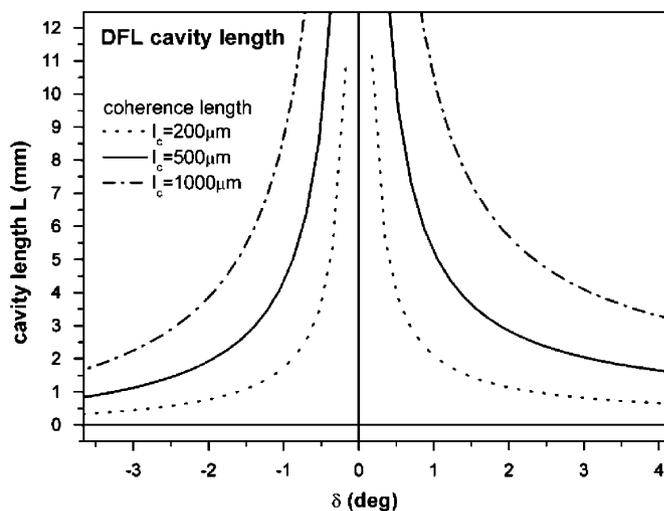
Fig. 2. Length of the interference pattern  $L$  as a function of  $\delta$  for different  $l_c$ .
