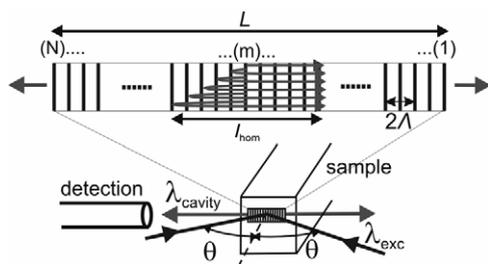
Fig. 1. Top: distributed mirror, used in the model calculation. Amplifying/absorbing material is separated from the mode-selective system. Bottom: DFL experimental setup.
