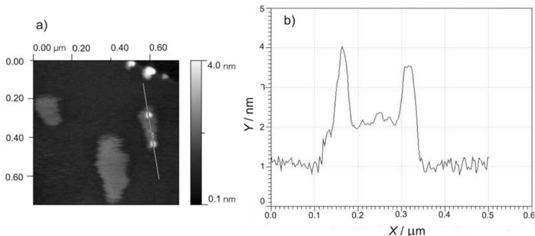
**Fig. 1.** (a) AFM image of  $750 \text{ nm} \times 750 \text{ nm}$  area of HOPG surface with several Si nanocrystals. (b) Profile taken along the white line. (The size of nanoparticles ( $\sim 2 \text{ nm}$ ) can be obtained from the height of peaks, while the lateral dimension of peaks is much larger than the real size of particles due to convolution with the AFM tip shape).
