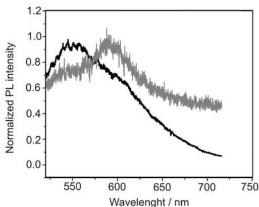
**Fig. 2.** PL spectra of several nanocrystal grains (passivated with  $\text{SiO}_2$ ) in L929 cells (grey line) and in ethanol (black line). Excited with  $325 \text{ nm}$  from a continual wave Argon ion laser.
