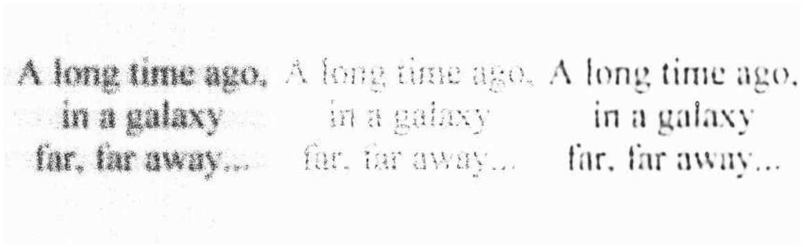
Figure 5.6: An example of ray-tracing of the non-astronomical artificial source in infinity. We use the astronomical LE mentioned in Section 4.2 with the pixel size of 50 \times 50 \mu\text{m}^2 . Result of the ray-tracing is on the left. It was processed using the standard Lucy-Richardson method with an automatic noise estimation and no threshold deviation of the result from the image. The result after 20 iterations is in the middle. The result after 20 iterations of the Multiresolution version of the Lucy-Richardson method with automatic noise estimation is plotted on the right image. The simulation is performed relatively deep inside the FOV of the optics, hence we can assume that the system is shift invariant.
