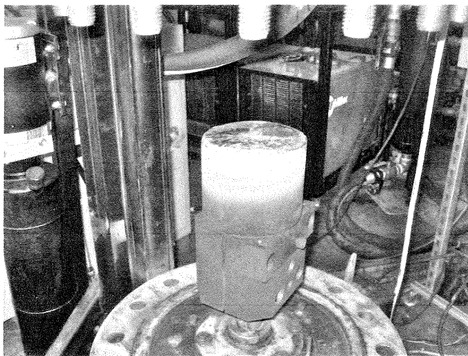
Figure 6: A view of the scorched carbon cathode following test 3.
